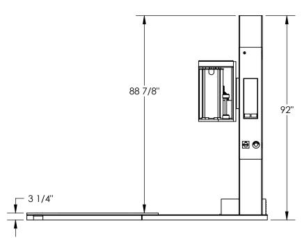
\*115V SUPPLY VOLTAGE; INCLUDES 12' LONG POWER CORD WITH NEMA 5-15 PLUG \*10A AT FULL LOAD
